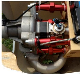
6. Connect the two remaining spark unit plugs (RPM and supply), at the injection unit plugs. Connect the last at the valve position sensor;
