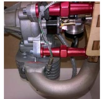
5. Connect the pick up sensor to the control unit and lock it on one of the engine mount with clamp. Do the same with the air sensor cable;
