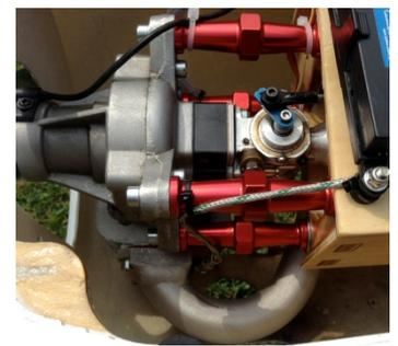
6. Connect the two remaining spark unit plugs (RPM and supply), at the injection unit plugs. Connect the last at the valve position sensor;
