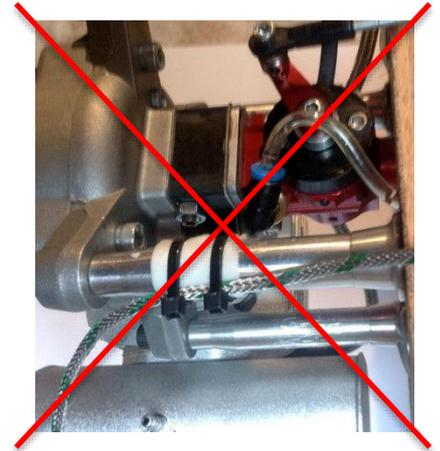
9. Connect the other end of the tube with the SMC valve installed on the injection unit;
